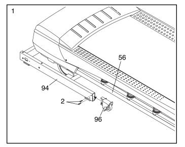
Pull the Upright Wire (81) and the Base Ground Wire (28) through the indicated hole in the Base (94).
