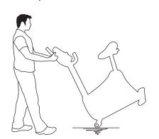
**RECUMBENT BIKES**: firmly grasp the steel portion of the rear stabilizer tube, carefully lift and roll on the transport wheels.
