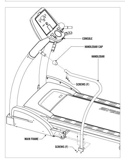
\*NOTE: The right handlebar side cap is marked with "R" on the side of the cap and the left handlebar side cap is marked with "L" on the side of the cap.
